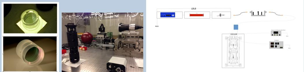
**Figure 3:** The FP etalons: optical (above) & infrared (bottom) (left). The working bench (middle).; Drawing of the all set up (right).
