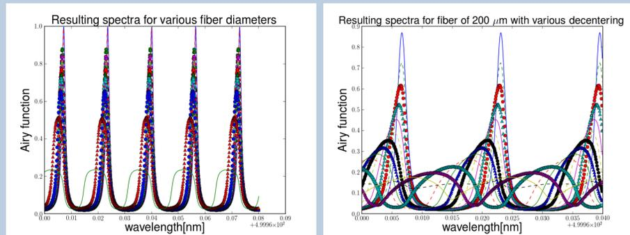
**Figure 1:** Simulation of transmission spectra of a Fabry Perot for different fiber diameters (50, 100, 200, 210, 220, 230, 240, 250, 260, 270, 280, 290, 300, 400, 600  $\mu\text{m}$ ) assuming the centered on the optical axis of the FP (left).; Simulation of transmission spectra of Fabry Perot assuming a fiber of 200  $\mu\text{m}$  with these decentering 20, 100, 150, 200, 250, 300, 350, 400, 450, 500, 600, 700, 800, 1000  $\mu\text{m}$  (right).
