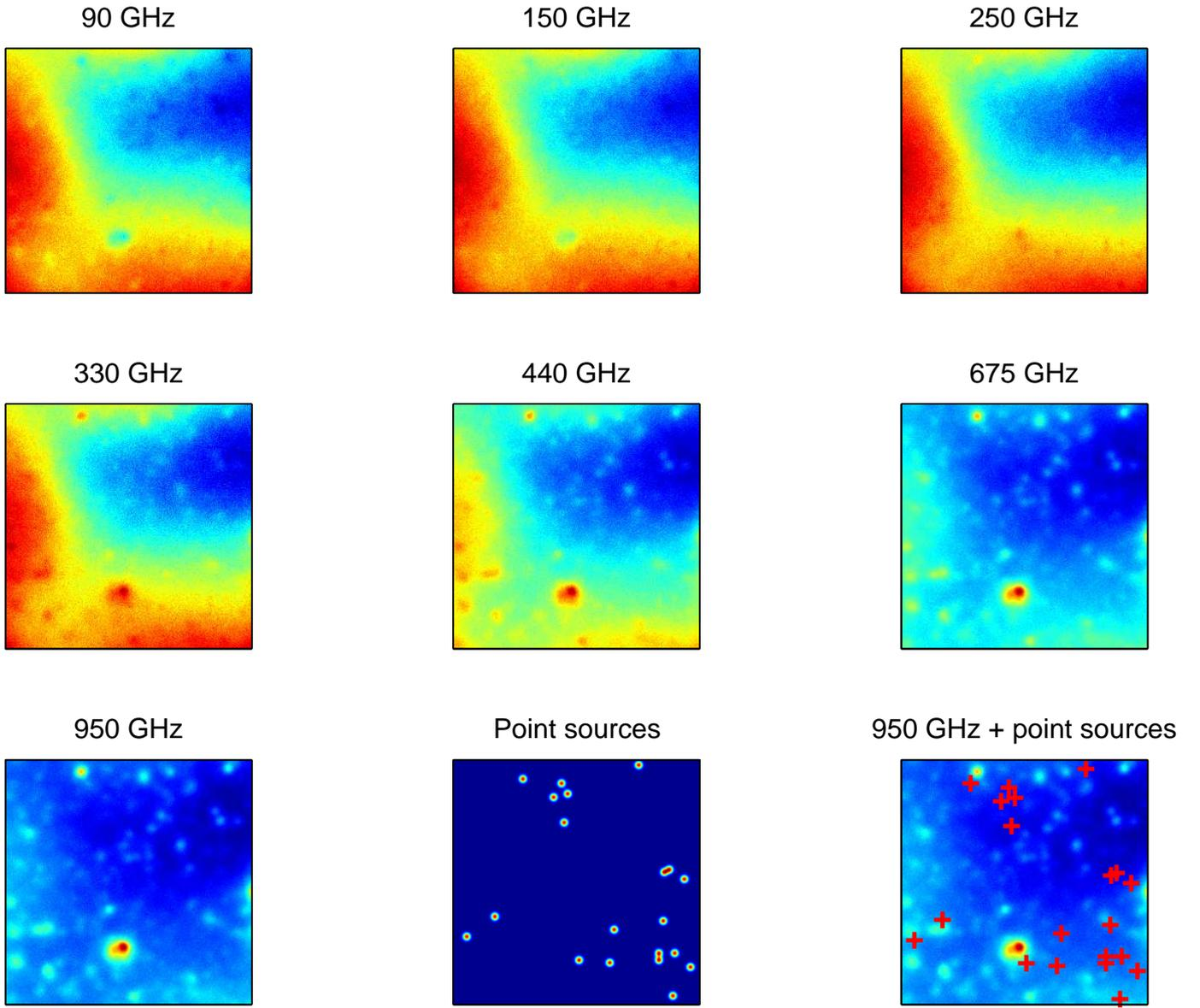
**Fig. 4.** Noisy version of the maps in Fig. 3. Noise is Gaussian-white with standard deviation set to 0.12 time the standard deviation of the values in the corresponding noise free maps. All of the point sources have the same intensity set to 1.7 times the standard deviation of the noise. The two bottom-right panels show the simulated point sources and their position on the 950 GHz map, respectively.
