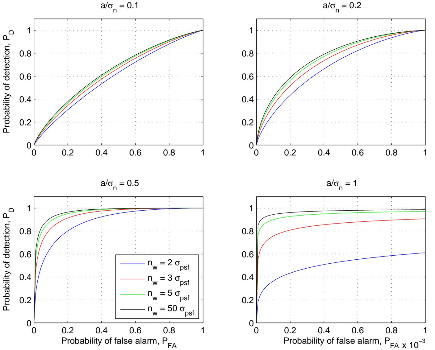
**Fig. 2.** Relationship between the *probability of detection*,  $P_D$ , vs. the *probability of false alarm*,  $P_{FA}$  for the case shown in Fig. 1 but for different values of the ratio  $a/\sigma_n$ . Note the different scale used for the abscissa in the bottom-right panel.
