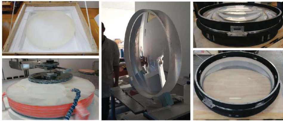
Figure 14: Current Status of the MOONS (ESO) Field Corrector lenses at Officina Stellare where they are being manufactured and integrated in the Field Corrector barrel.
