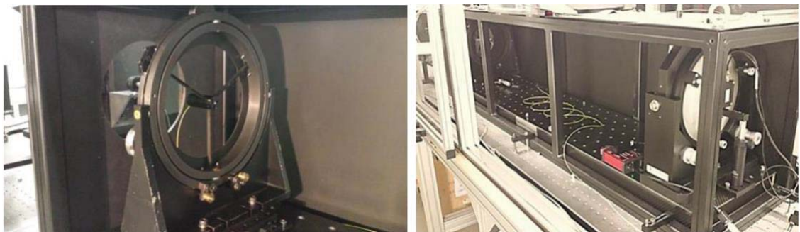
Figure 18: The PLATO (ESA) White light collimator during integration. Detail of the fibre holder (left) and mirror gimbal (right).
