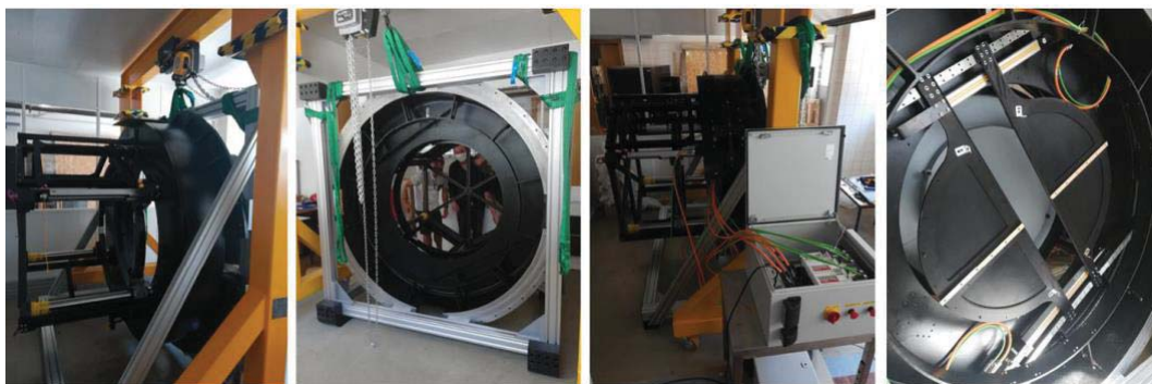
Figure 15: The MOONS (ESO) Rotating Front End during integration and tests of the retraction and screen mechanisms.
